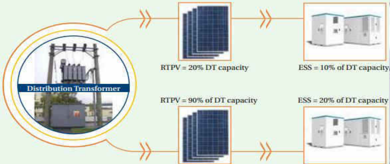
ESS requirement (as percentage of DT capacity) in Metro Growing Scenario with different solar PV penetration (IESA Analysis)
