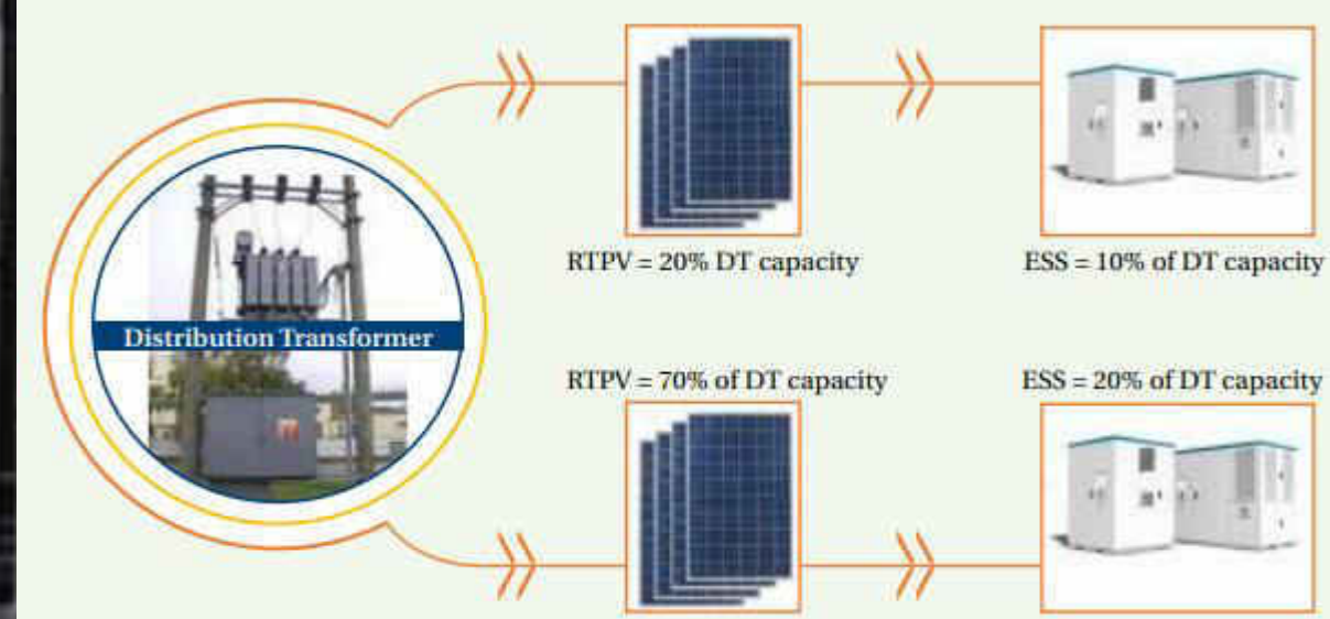
ESS requirement (as percentage of DT capacity) in Metro Saturated Scenario with different solar PV penetration (IESA Analysis) 33
