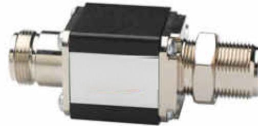
Arrester flashover voltage should equal twice the peak line voltage. Example in a 50 ohm line with 50W transmitter, peak voltage = 70.7V. Minimum recommended gas arrester BV = 140V. Nearest value = 230V. Surge rating should be 20KA for an 8/20us impulse.
